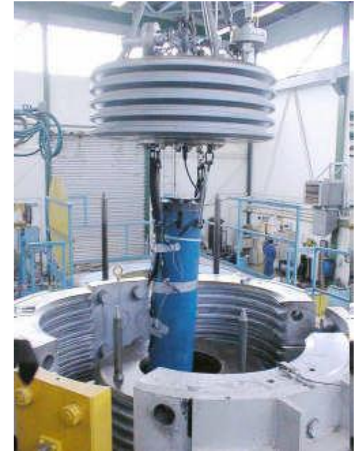
Hyperbaric tanks for resistance test to high pressure
