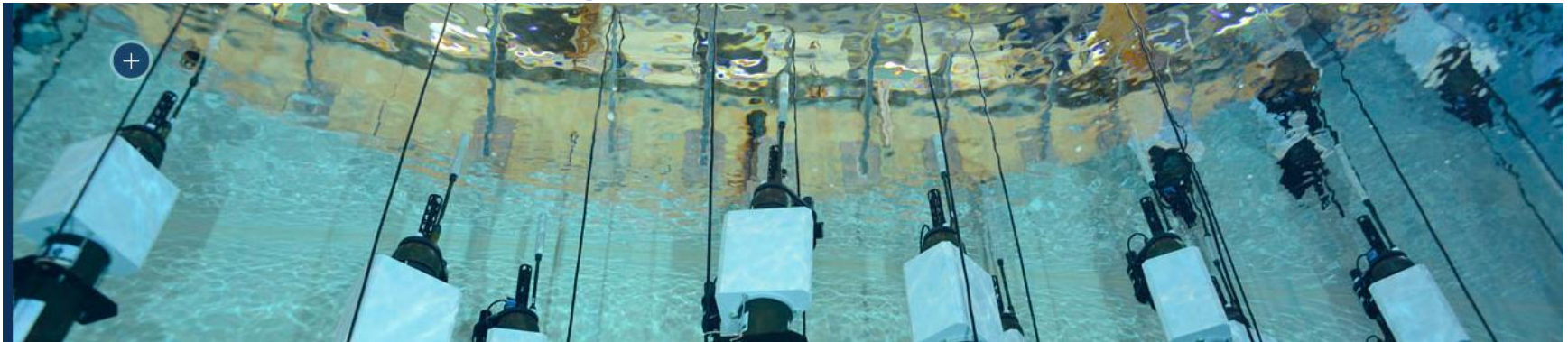
Profiler Bio cycling tests in deep basin
