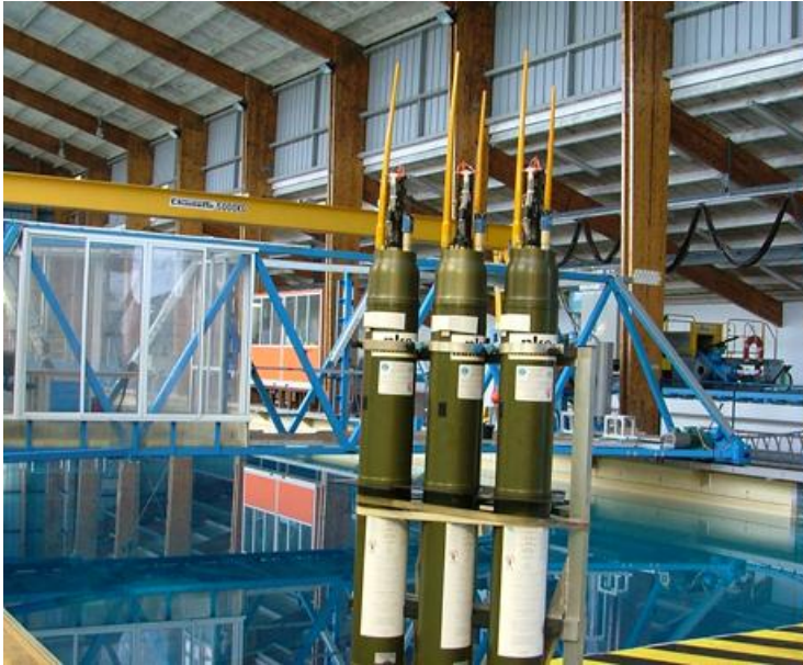
Profiler Bio cycling tests in deep basin
